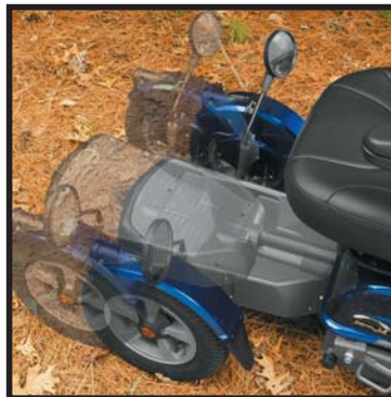
Power extendable front end allows custom fit for every user and added stability.
