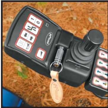
Key protected control box
